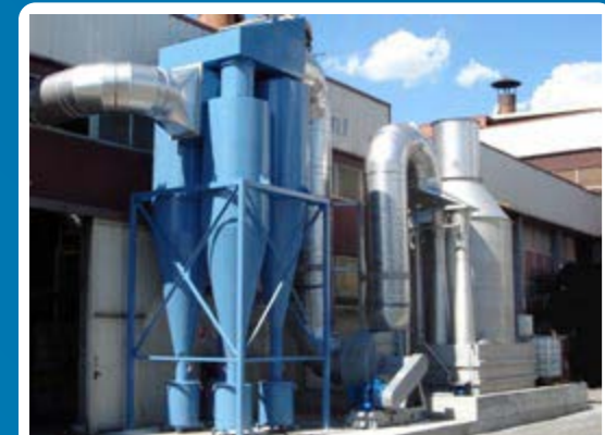
DUSTS AND AMINES TREATMENT FROM COLD-BOX CORE-SHOP DEPARTMENT ABBATTIMENTO POLVERI E AMMINE DA REPARTO ANIMISTERIA COLD-BOX
